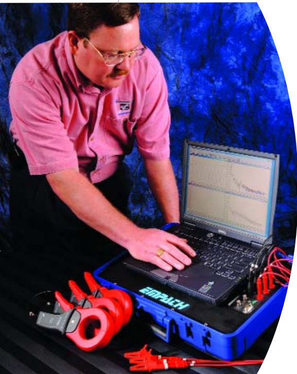
Portable Motor Current Signature Analysis system provides early rotor failure detection.
